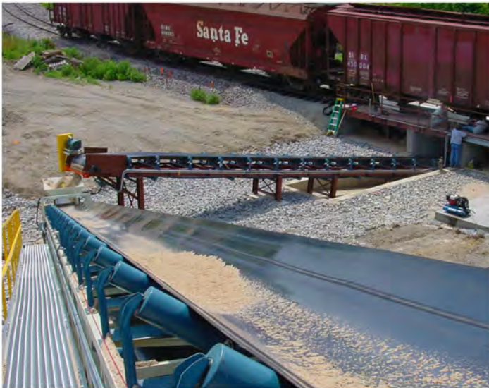
A shallow pit design rail car un-loader with a pit under the hopper, feeders and collecting conveyor. The collecting conveyor feeds a 100' radial stacker. These systems are typically designed to unload at 500 TPH. The track hoppers are sized so that the rail car does not need to be moved while emptying.
